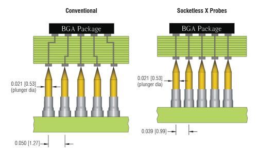
The X Probe Socketless Series comprises two parts: a test probe and a termination pin. The probe is designed around our patented rolled probe tube design with a modified interconnect receptacle on the bottom. This interconnect receptacle increases the tube length while all other aspects of the probe are the same. The interconnect receptacle receives the precision interconnect pin located at the top of the termination pin.
