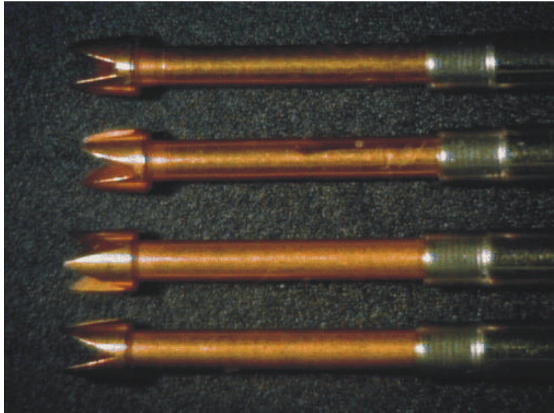
Comparison of two gold-plated BeCu plungers (top) and two steel plungers after running 500,000 cycles against a contact surface angled at 30°. There is no practical difference in plating wear or electrical performance between the two materials.
