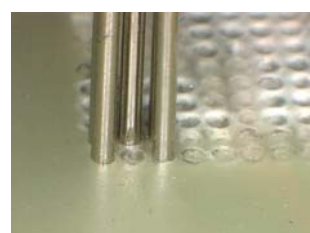
Broken off tube is completely removed from the drilled hole.
