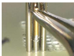
Using tweezers pull straight up on the soldered plunger thereby removing the broken tube.
